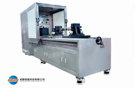
The actuator test bench meets the test requirements of various conventional linear actuators of the C919 aircraft, including the main landing gear retractable actuator, the main landing gear lower lock actuator, the main landing gear door actuator, and the nose landing gear. Retractable actuator, front landing gear lower lock actuator, front landing gear door actuator, ground spoiler
